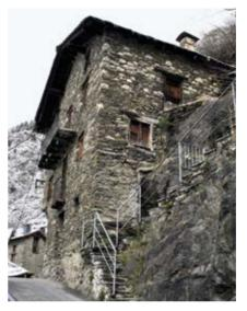
A family house typical of the traditional 18th century Andorran family homes. It has three floors and a loft, faces the sun and is excavated into the rock. It is built in granite and slate and has a ridge roof. The top floor is balconied, to take all possible advantage of the sun's warmth. Here the people living in the house came to take the sun, hang out the laundry and dry fruit. The iron balconies were a sign of wealth. They still survive.
